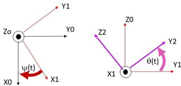
$$\overrightarrow{V(P/R_0)} = \left\{ \frac{d\overrightarrow{OP}}{dt} \right\}_{R_0} = \left\{ \frac{d\overrightarrow{OG}}{dt} \right\}_{R_0} + \left\{ \frac{d\overrightarrow{GP}}{dt} \right\}_{R_0}$$
